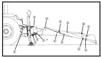
Figure 6 - Lubrication Points for Model 665H
